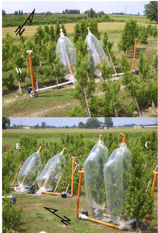
Fig. 1. Trees of the asymmetric orchard enclosed in whole plant chambers during the gas exchange measurements.
