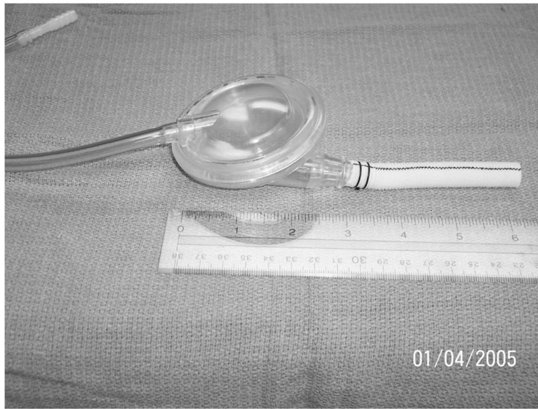
Figure 1. Photograph of a 40-ml counterpulsation device (CPD). The CPD sac (1) fills with 40-ml blood volume during ventricular systole and empties during ventricular diastole through a single, valveless cannula (2). The diaphragm is pneumatically driven by controller through an air line (3).
