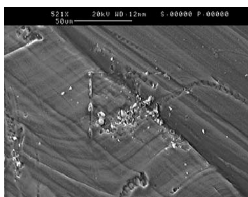
Figure 4 The concave wall structure after mixture of detergent and Escherichia coli cultured; surfaces are part of the biofilm formation.
