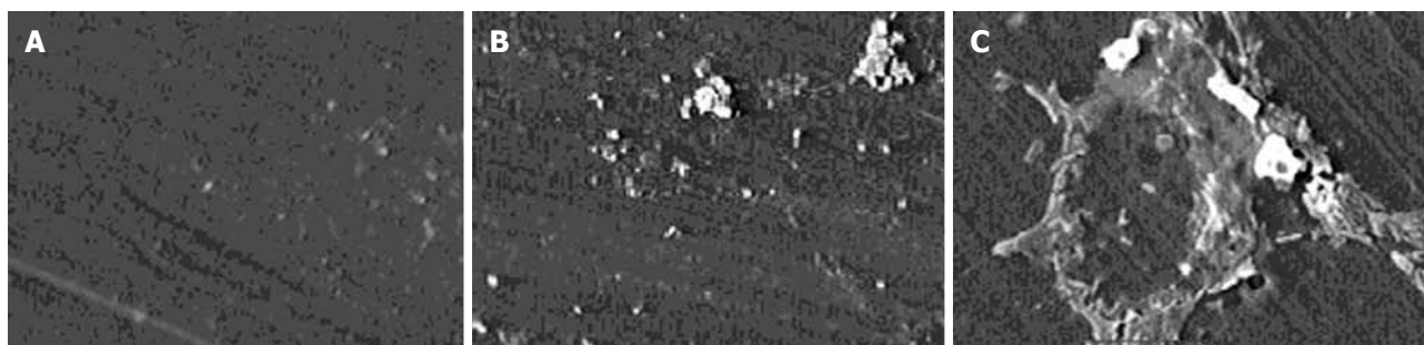
Figure 5 The concave wall structure after non-enzyme detergent (A), enzyme-containing detergent (B), and sterile distilled water (C) washing. A: No obvious biofilm residue; B: Massive biofilm structure residue; C: Relatively large biofilm attached to bacterial biomass, respectively.
