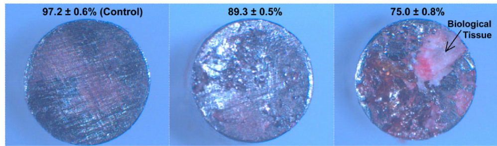
Fig. 9. LENS processed porous Ti6Al4V implants after 16 weeks implantation in rat intramedullary defects.
