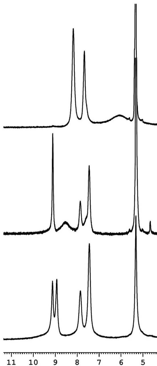
Figure 4. 1 H-NMR spectra recorded in CD 2 Cl 2 . Top - (F 8 )Fe(NO), RT. Middle - (F 8 )Fe(NO) at -80 °C. Bottom - of (F 8 )Fe(NO) 2 at -80 °C. The peak at 5.32 ppm is CD 2 Cl 2 .
