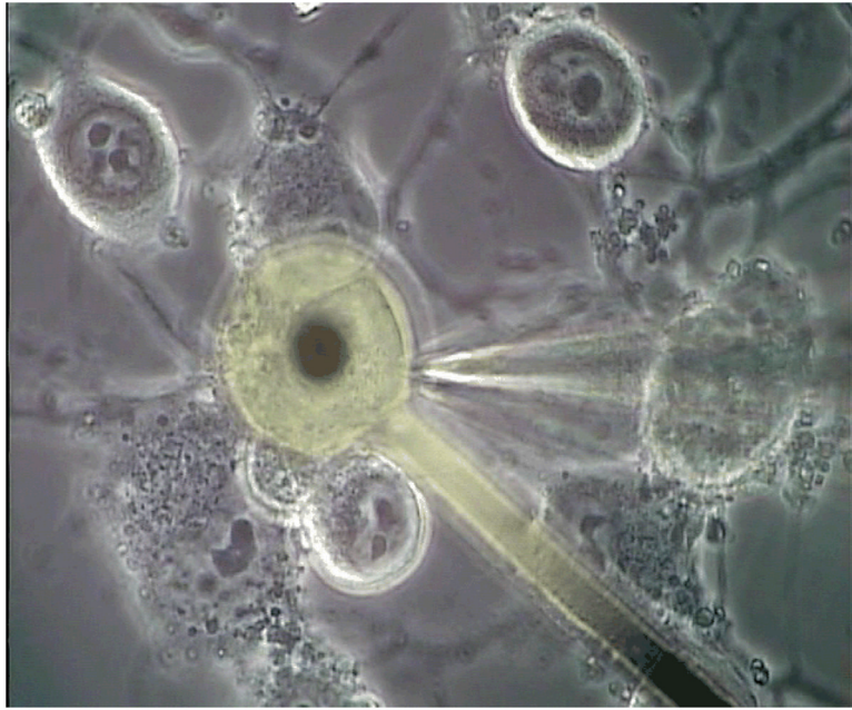
Figure 2. Micrograph of a neuron that is over an extracellular microelectrode while simultaneously being stimulated with bandlimited Gaussian white noise through a glass patch-clamp micropipette.
