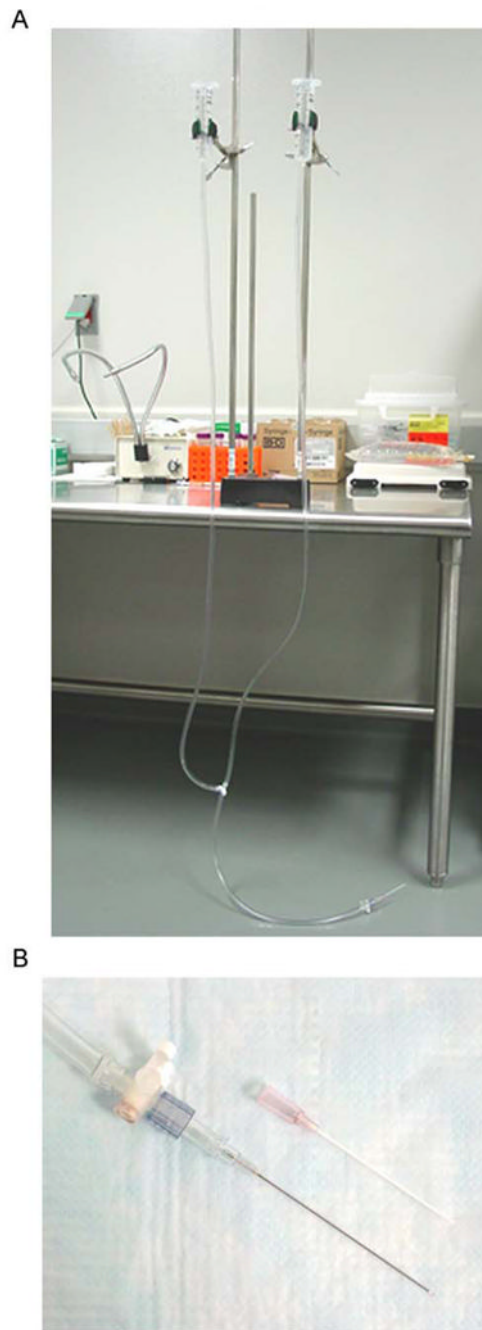
Figure 2. Photographs of an in situ perfusion-fixation apparatus. A: complete apparatus; B: close-up photo of over-the-needle catheter (with catheter removed) attached to stopcock and tubing.
