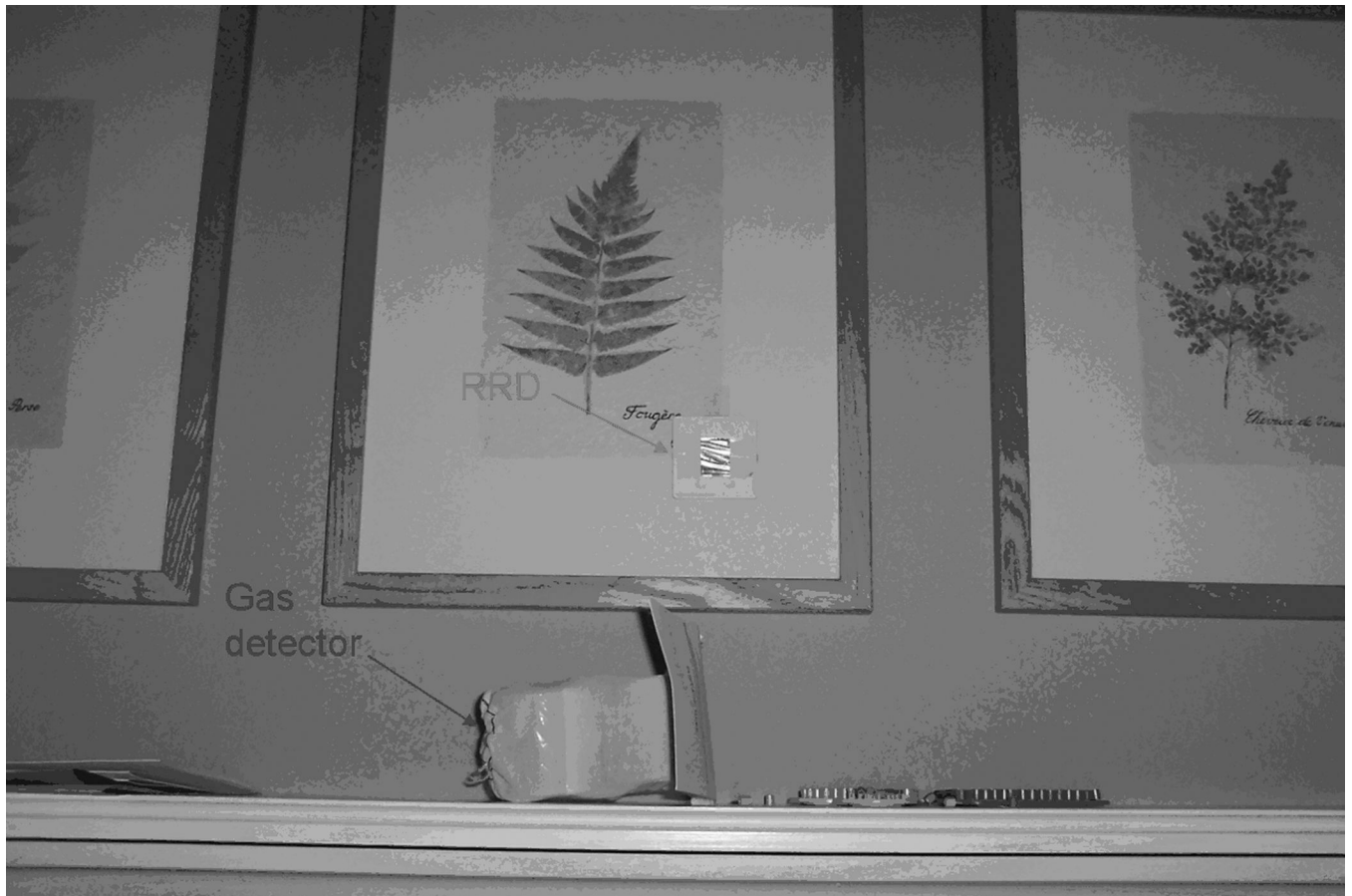
Figure 3. The glass-based RRD and radon/thoron gas detectors are simultaneously exposed for 90 days in a selected room
