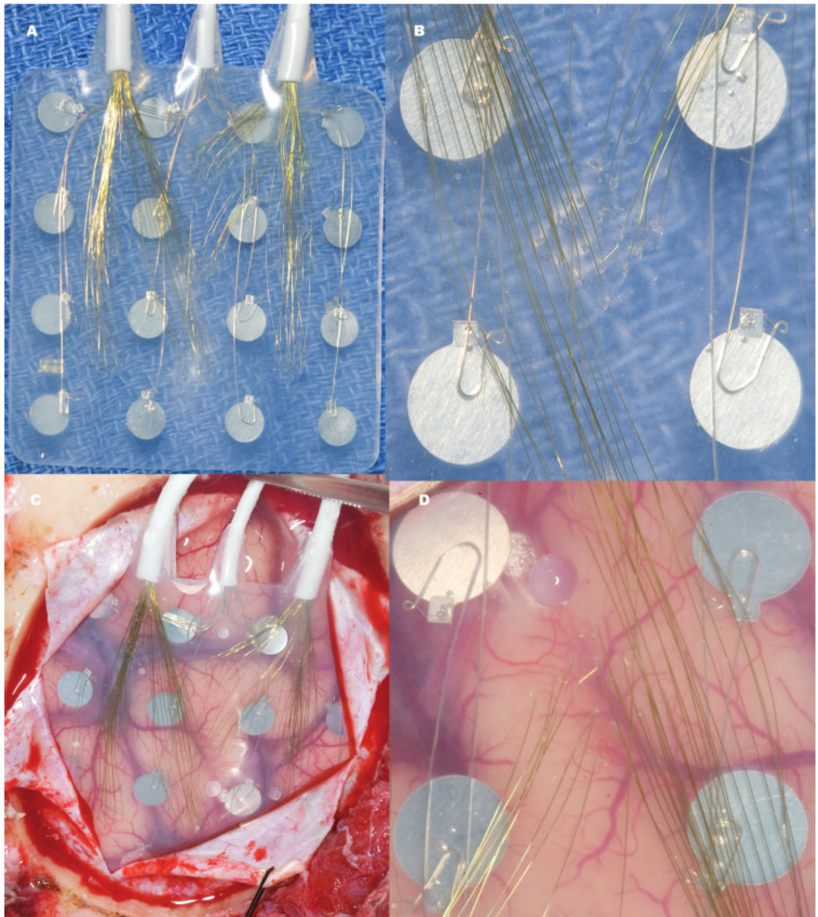
Fig. 2. Depictions of the hybrid grid for intracranial monitoring. A. Low magnification view of hybrid 4 \times 4 grid prior to implantation. B. High magnification view of the grid subunit. Note how 4 macroelectrodes surround a diamond-shaped and centered 4 \times 4 grid of microwires. C. Low magnification view of implanted grid in a patient. D. High magnification view of grid subunit over human cortex. note the improved spatial resolution of microwires compared to macroelectrodes.
