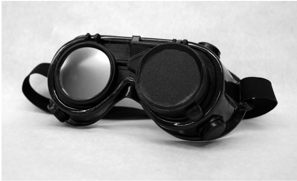
Figure 2. Degraded vision goggles: welding goggles with the left eye occluded and a theatrical lighting gel in the right eye to impair vision.
