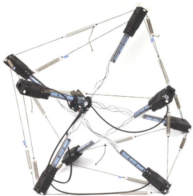
Figure 3. A tensegrity robot consisting of four strut modules and 16 strings. The strut modules consist of servo motors connected by clear plastic tubes which contain batteries and wiring.
