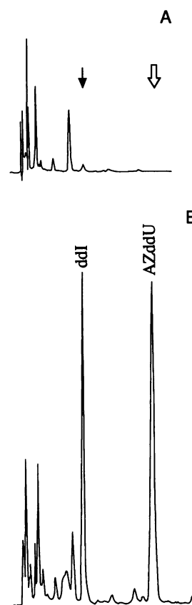
FIG. 1. Chromatograms obtained from HPLC analysis of ddI in a monkey plasma blank (A) and in a sample obtained from animal D1 3 h after i.v. administration of 20 mg of ddI per kg (B). Black and white arrows indicate retention times of ddI and AZddU, respectively.
