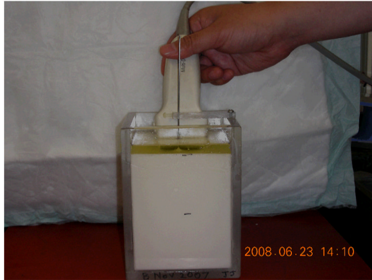
Fig. 2. A photograph illustrating data acquisition setup for the phantom experiment under freehand scanning. An imaging plane (typically 3-mm away from the needle electrode) is chosen to maximize the cross-sectional area of the spherical lesion without introducing reflection from the metal
