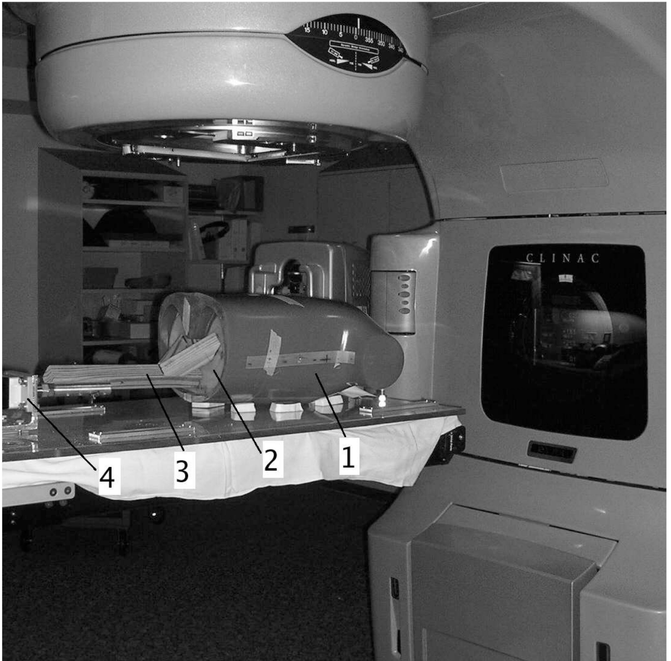
FIG. 12. A picture of the movable phantom: 1. the phantom; 2. the diaphragm; 3. the wood connector; 4. the actuator.
