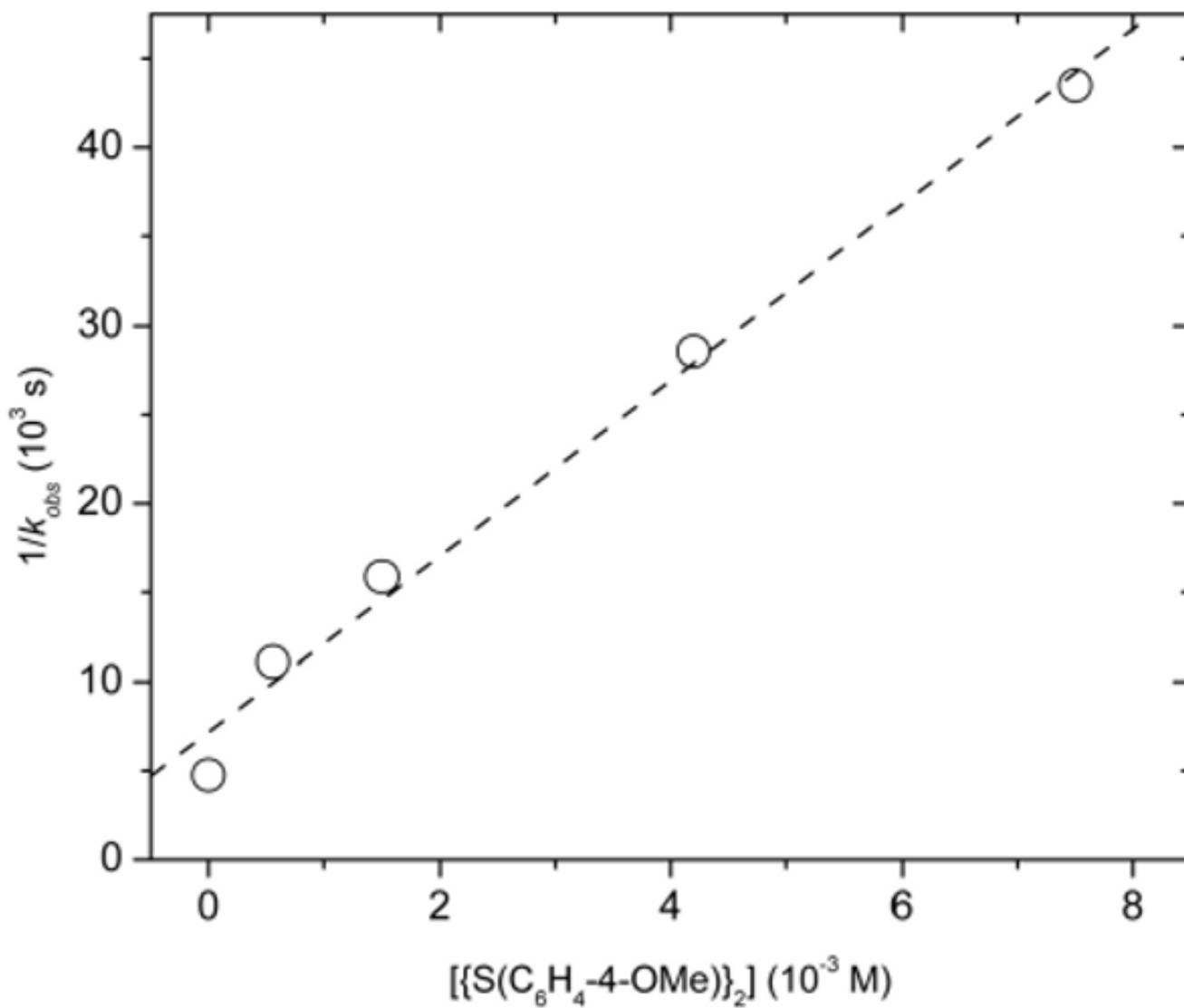
**Figure 3.** Plot of  $1/k_{\text{obs}}$  vs  $[\text{S}(\text{C}_6\text{H}_4\text{-4-OMe})]_2$  for the reaction of bis-thiolate complex **7** with 4-bromotoluene.
