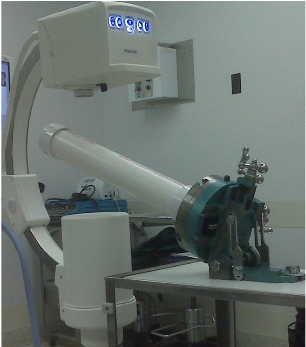
Figure 1. Custom cross-slide rotary table used to position specimens.
