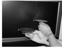
Figure 1. Comparison of visible smoke between a charcoal-based smokeless mosquito coil (Lanju Smokeless coil appearing in black) and a sawdust-based conventional mosquito coil (Bison coil appearing in gray)
