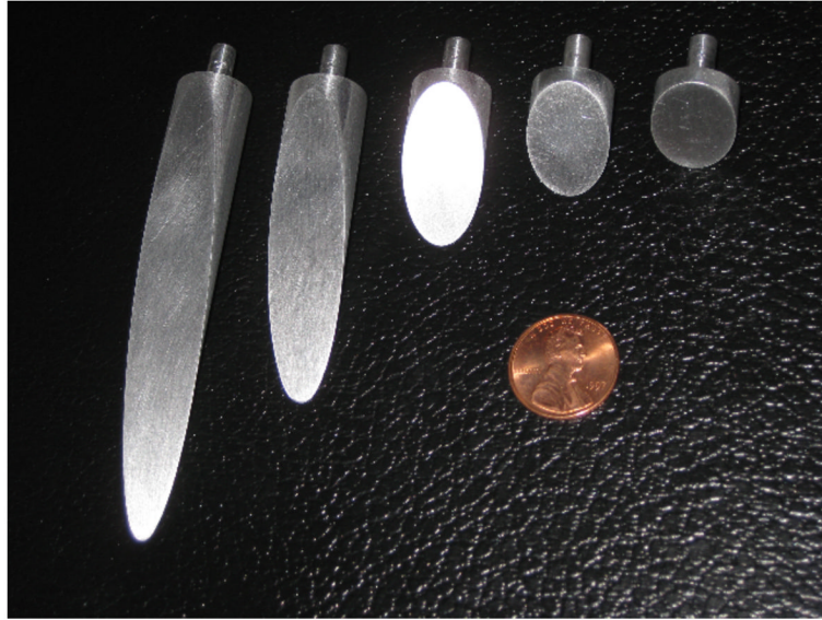
Fig. 4. Scaled needles of \text{\O} 1.5 \text{ cm} used to understand the interaction between the needle tip and medium. Needles of various bevel angles ( 10^\circ , 15^\circ , 30^\circ , 45^\circ , and 60^\circ ) were used in the study.
