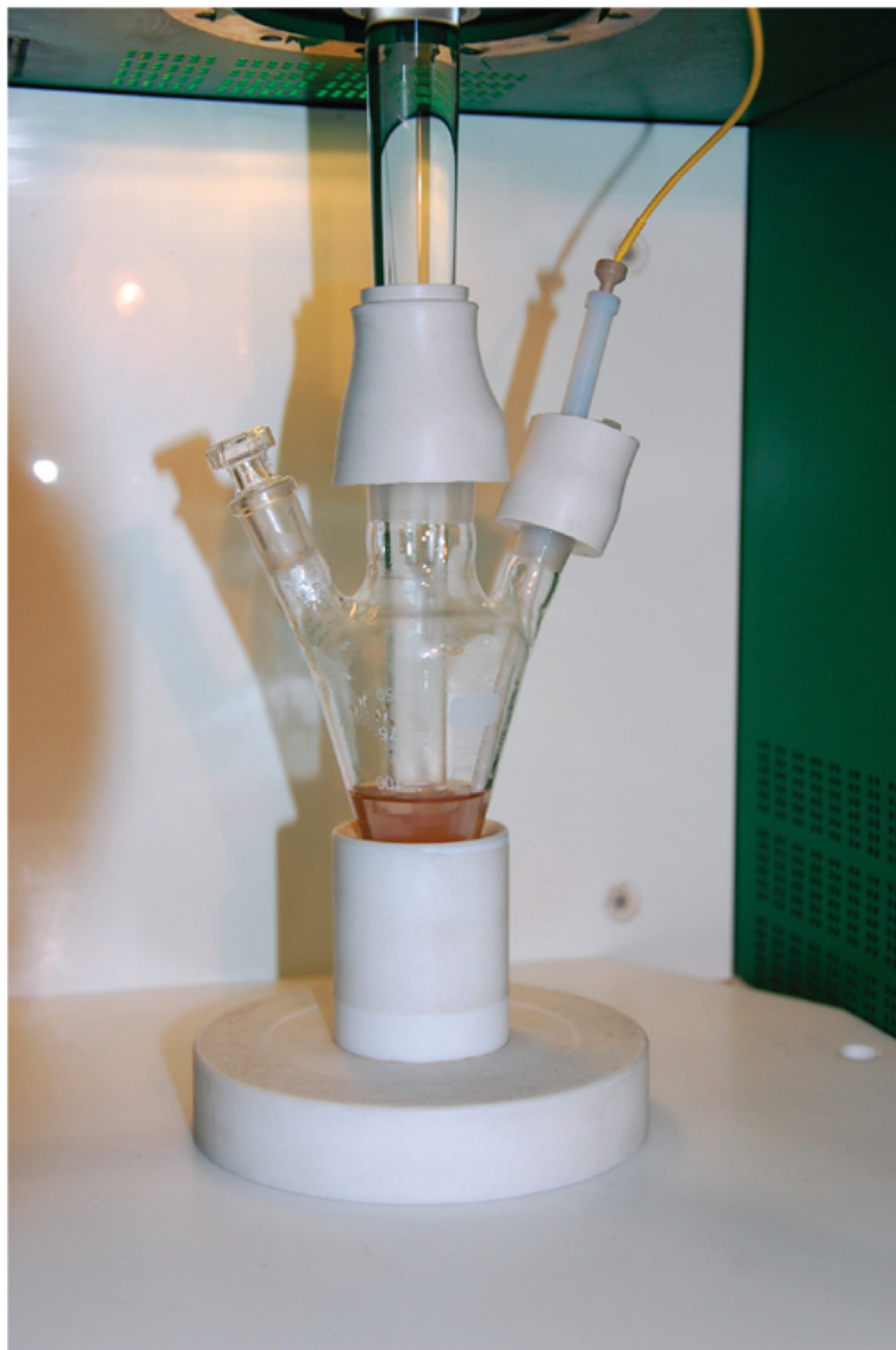
Figure 2. General setup for simultaneous US/MW irradiation.
