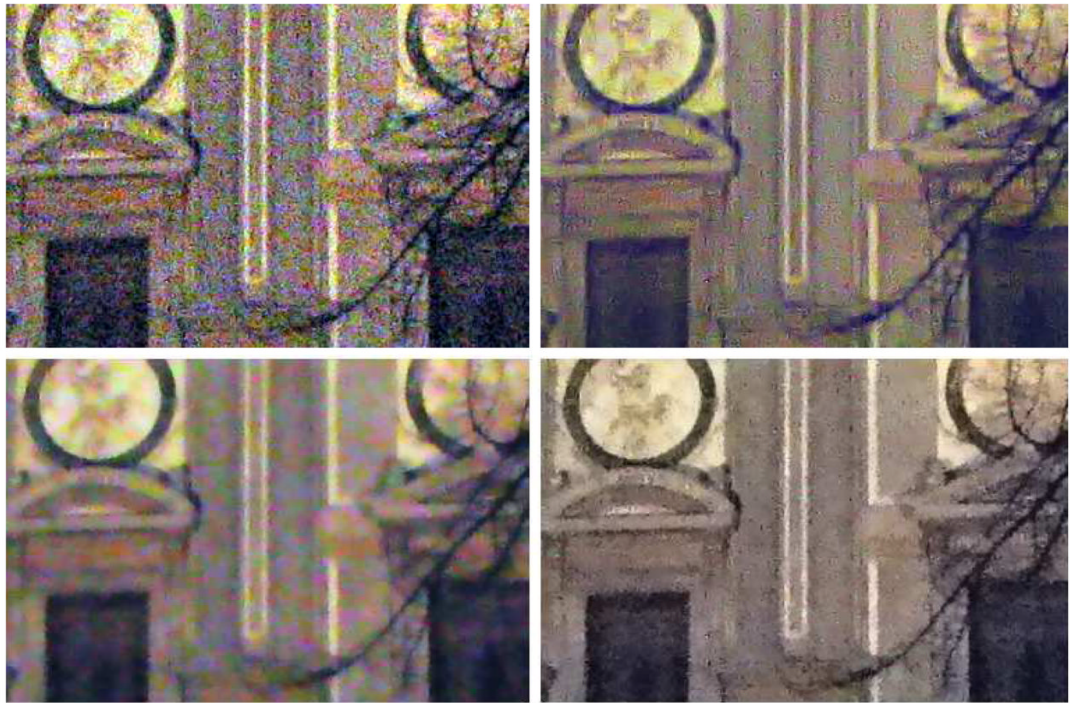
Figure 6. (a) Input image obtained from 23 (b) The BLS-GSM result obtained from 23 (c) The bilateral filter 3 result (d) Result of the proposed method. For the bilateral filter, \sigma_d = 1.8 , \sigma_r = 10 \times \sigma_n , and the window size is 11 \times 11 . For the proposed method, \sigma_d = 1.8 , \sigma_r = 3 \times \sigma_n at each level, the window size is 11 \times 11 , and the number of decomposition levels is (1, 4, 4) for the ( L , a , b ) channels, respectively. The wavelet filters are db8 in MATLAB. The noise parameter \sigma_n is estimated using the robust median estimator.
