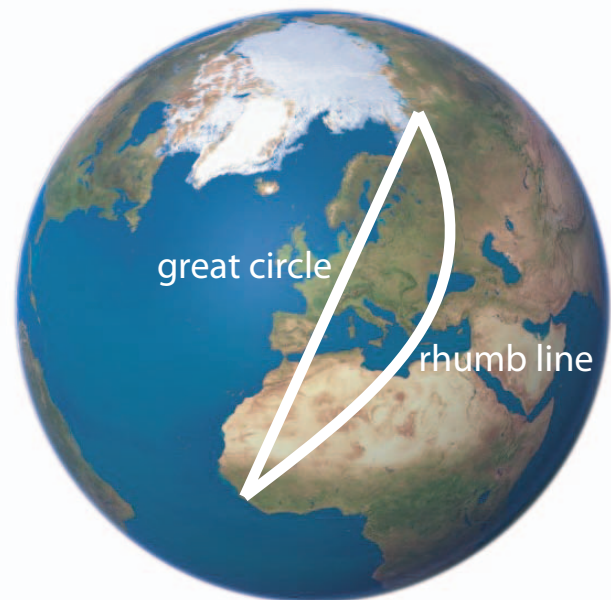
Figure 5. Illustration of how the great circle (orthodrome) and rhumb line (loxodrome) differ between two locations on the spherical globe. The rhumb line is a constant compass course from the point of departure to the destination, while the great circle involves a continuous shift of the compass direction. On the global view shown here, great circles appear as straight lines if passing through the centre. doi:10.1371/journal.pbio.1000362.g005
