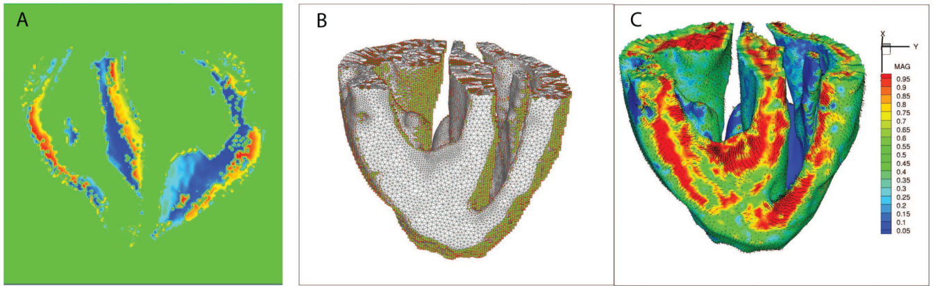
Figure 5. Automatic mapping of 3D cellular information. Data is the direction vector of the myofibers in a sheep heart, as revealed by diffusion tensor MRI. A) the direction and magnitude of the vector in a voxelated MRI dataset. B) The overlap between the unstructured grid (grey) and the voxel grid (green). Note that the algorithm is very tolerant of small geometric mismatching. C) The vector field mapped onto the unstructured grid.
