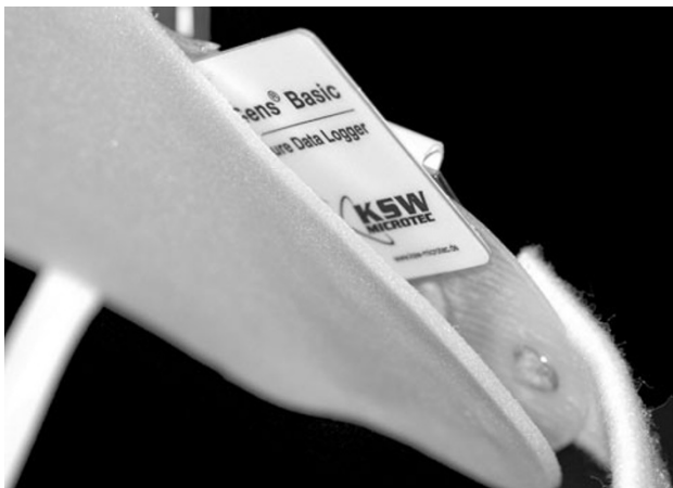
Fig. 2 The data logger (dimensions 86 \times 54 \times 1\text{-mm} ) is sandwiched between the 1.5-mm-thick pelvic base and a 4-mm-thick extra layer of gel foam, which is in direct contact with the patient's slip
