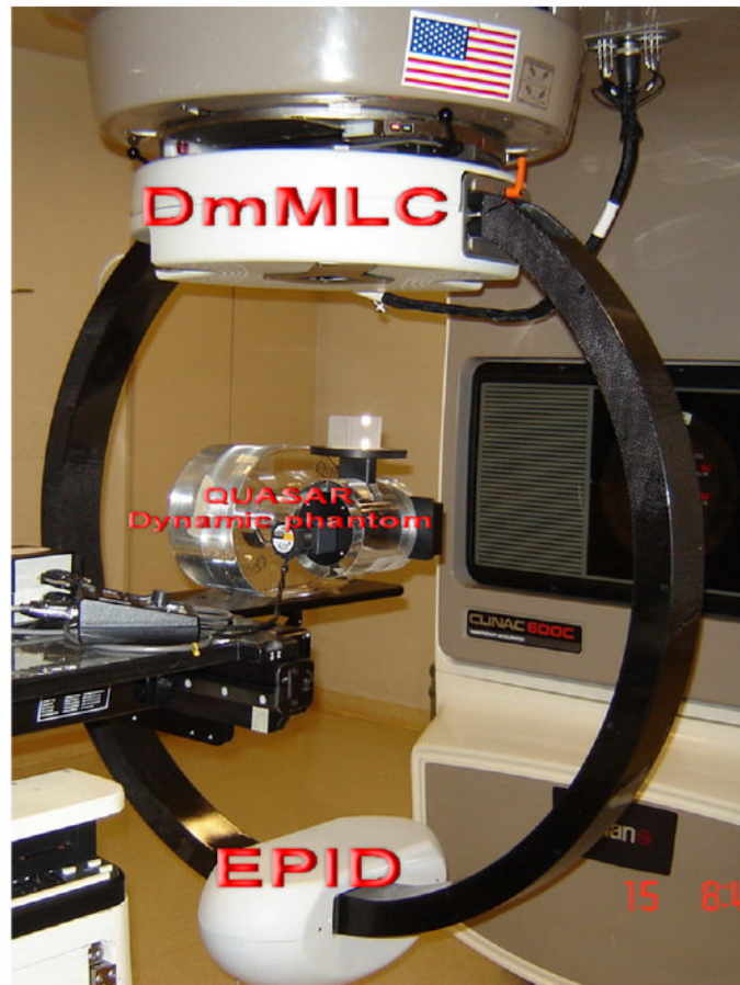
Figure 1. Experimental setup showing the TrackBeam dual-layer micro MLC (DmMLC) and EPID integrated to the CLINAC 600 linac. The QUASAR dynamic phantom set on the linac couch is also shown.
