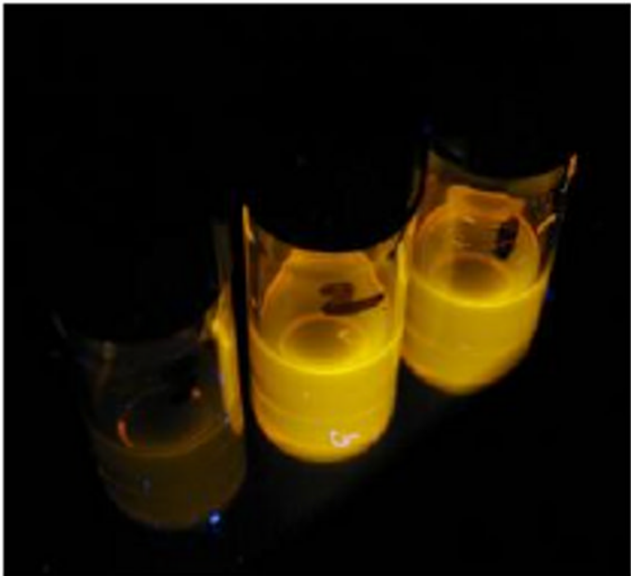
Figure 8. Luminescence of 5 \mu\text{M} CdSe QDs in toluene in the presence of (from left to right): carboxylic acid nitroxide 3 (2500:1 moles of nitroxide 3 :QDs), TEMPO (2500:1 moles of TEMPO:QDs), and no additive upon illumination with a TLC lamp at 366 nm.
