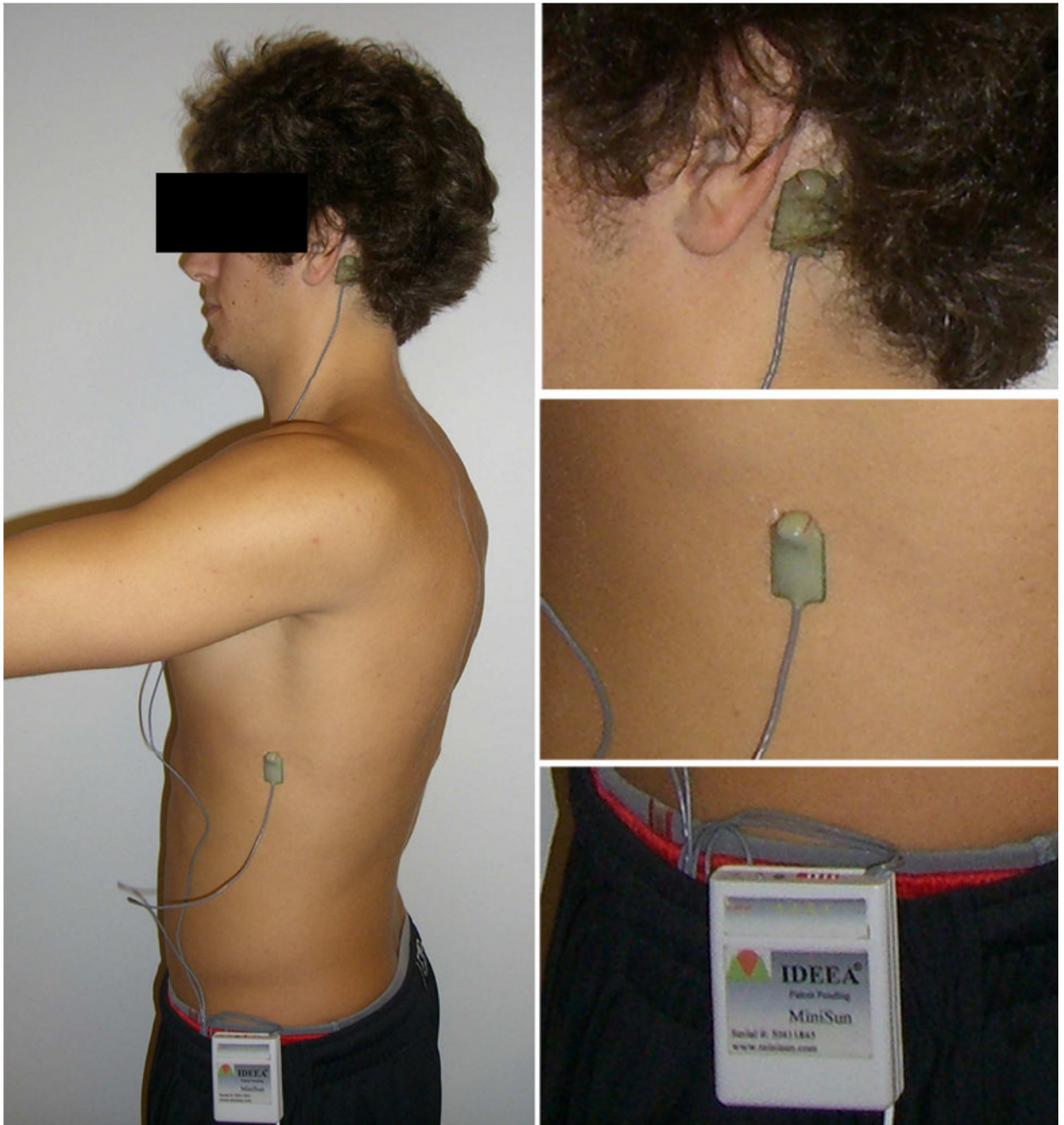
Figure 1. Subject wearing the WASP unit. Data sensors attached with medical adhesive to the mastoid process and the intersection of the 7 th rib and the mid-axillary line on the left side of the body.
