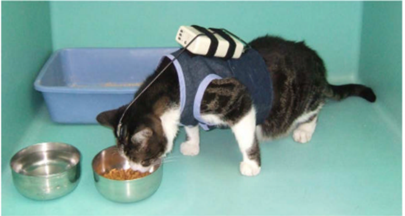
Fig. 6. Animal wearing the torso vest with the attached controller for bidirectional telemetry.
