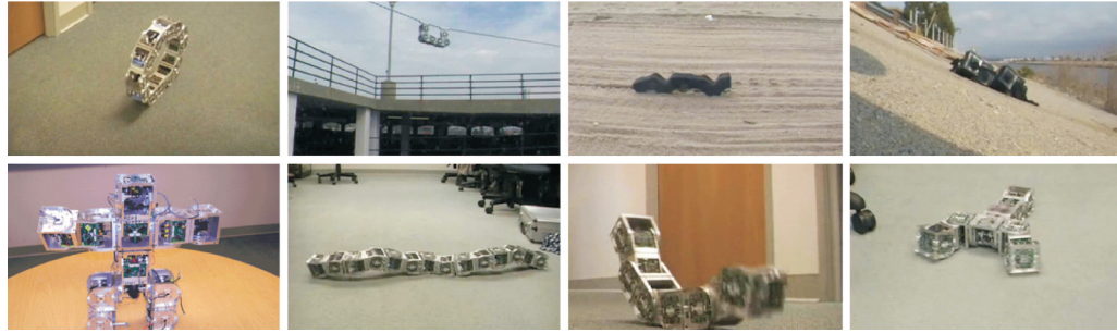
Fig. 9. Multifunctional examples of robotic stem cells based on SuperBot modules
