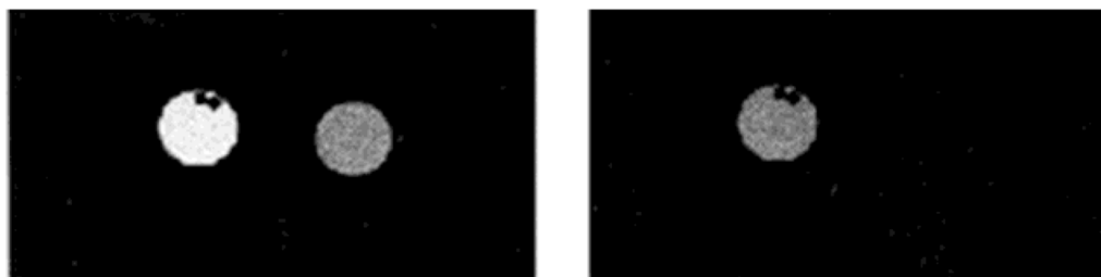
Figure 65. The spin echo images at 4.7 T and room temperature of a phantom containing Dy 3+ - 1 and Dy 3+ - 101 . Reference 314 . Copyright (2002); Reprinted with permission of John Wiley & Sons, Inc. 314
