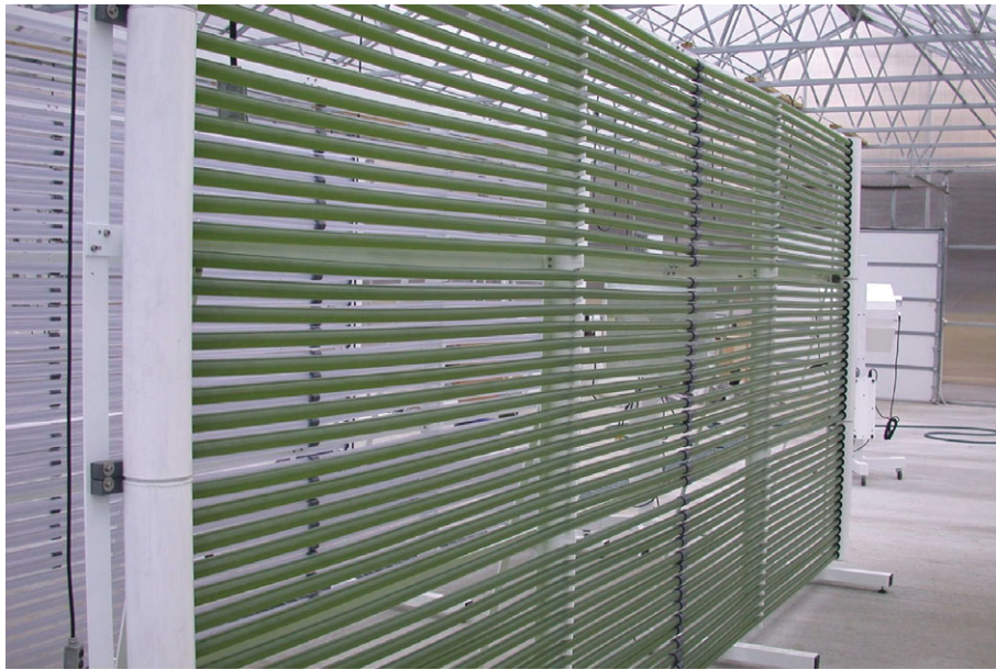
Figure 5. Tubular PBRs in operation. Such systems have a small path length ensuring high volumetric production coupled with a small footprint. Photograph courtesy of Varicon Aqua Solutions Ltd, UK.
