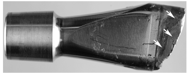
Fig. 3 The retrieved modular neck demonstrates fretting and corrosion damage (arrows) on the surface that had mated with the femoral stem.
