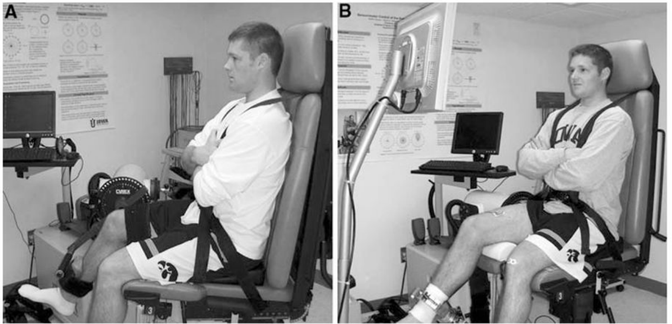
Fig. 1. A subject positioned on the test system for an isometric knee strength test (a) and EMG-contraction intensity testing (b)
