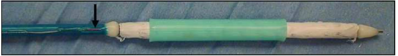
Figure 2. TAG device with integrated sensor coil. The arrow highlights the location of the sensor coil with the wire extending along its delivery catheter shaft.
