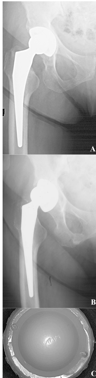
Figure 6. A-C. Anterior-posterior radiographs for case study 1, a Crossfire liner revised after 3.1 years. 1.5 months postoperative radiograph, (6A), and 3 years postoperative, (6B). After implantation, the liner rim, (6C), showed localized plastic deformation and whitening (oxidation index ~ 5.0 at the rim).
