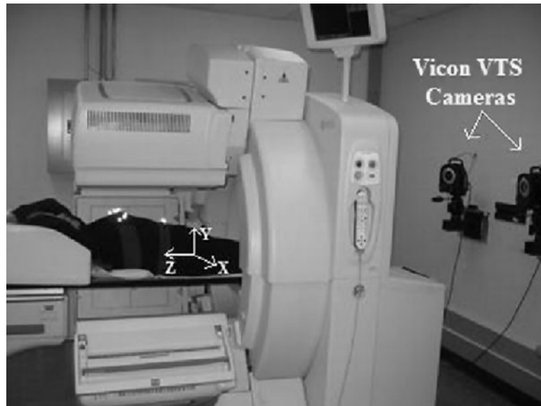
Fig. 1. SPECT and Vicon Visual-Tracking System (VTS) setup. Shown are two near-infra-red cameras mounted on the wall at the foot-end of the gantry. Three more cameras (not shown) are mounted on the wall at the head-end of the gantry. The retro-reflective markers on stretchy bands may be seen as bright spots on the chest and the abdomen of the subject. The coordinate system for the VTS as calibrated to the SPECT coordinate system is shown with X being lateral, Y vertical, and Z axial. The arrows indicate positive direction of the axes. The coordinate system of the projections is X' , and Y' .
