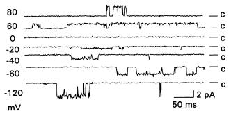
Figure 6. Single nonselective channel events. Cell-attached recording shows inward current events at  $-V_{pipet} < 0$  mV. Fc = 1 KHz; sampling = 5 KHz; and no software filtering.
