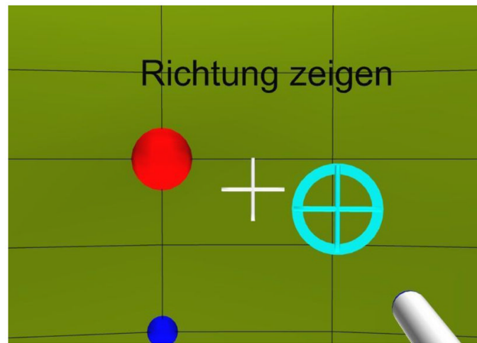
Figure 1. (color online). VE from the subject's point of view. The large (red) ball denotes the reference position. The small (blue) ball denotes the meridian. The (white) cross-hair represents the center of the display. The (white-shaded) cylinder in the right-bottom corner is the visualization of the manual pointer. The (cyan) circle with a cross-hair shows the projection of the pointer on the sphere. Instructions were presented at the top of the field of view ("Point to the direction" in this example).
