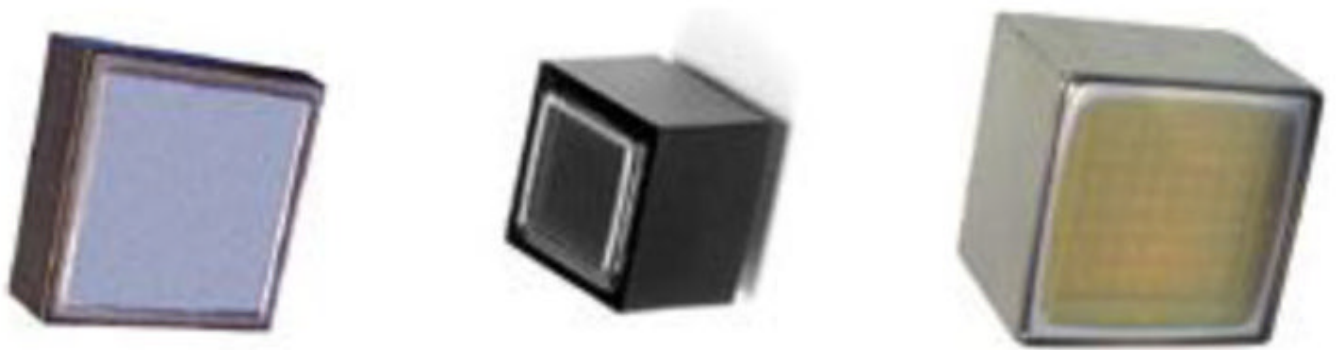
Figure 10. Examples of multi-channel PMTs from Burle (left), Hamamatsu (center) and Photonis (right). Such devices come in a variety of sizes with 4–256 channels and have been one of the key components in new PET detector designs.
