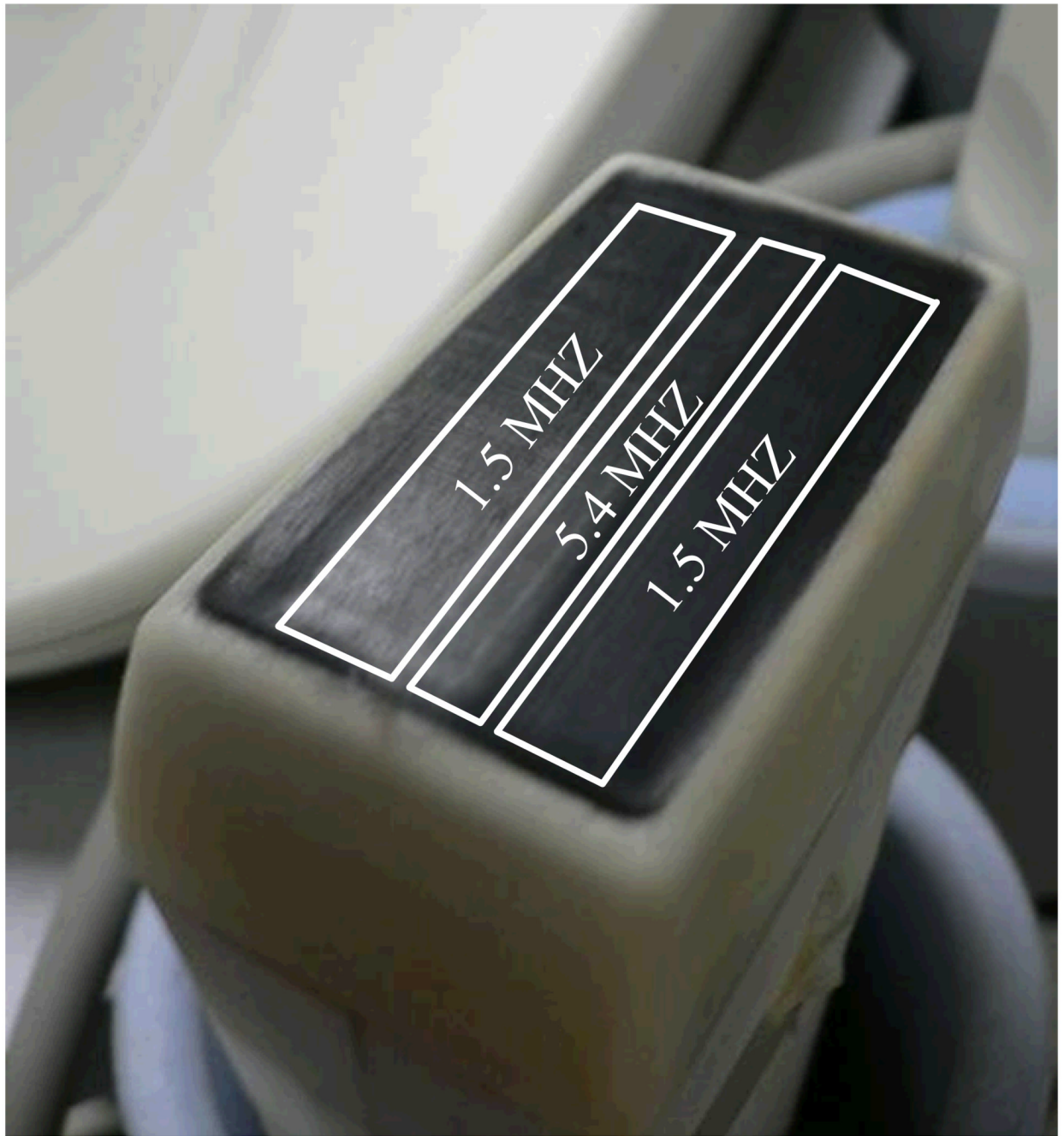
Fig. 1. Co-linear array transducer face with 3 individual arrays delineated: the center high frequency (5.4 MHz) array is surrounded on each side by low frequency arrays (1.5 MHz).
