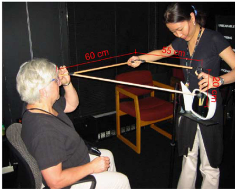
Fig. 1. Experimental setup for the reflected glare study for nighttime condition.
