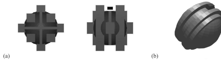
Fig. 8. Motion planning problems involving: a) moving a robot (black) from the north pole to the south pole. Multiple views of the geometry of the problem are shown (obstacles are drawn in lighter shades); and b) moving a robot along the corridor.
