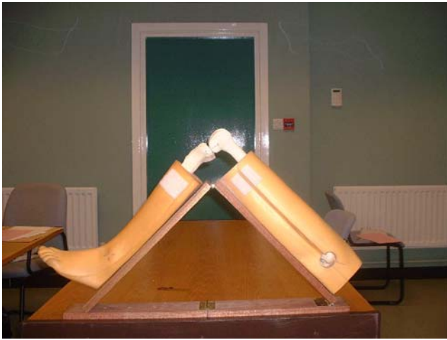
Fig. 4 Prosthetic limb used in accuracy testing
