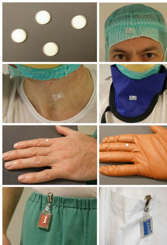
Fig. 1 Positions of the thermo luminescent dosimeters (TLDs) exposed to radiation during fluoroscopy. The TLDs were secured to the operating surgeon's forehead, the thyroid gland under and above the lead collar, on the second finger under the gloves, and on the third finger above the lead gloves in a standardised manner. Furthermore, a personal TLD was carried at the waist under the lead apron. The exact same lead apron and collar were used during all operations
