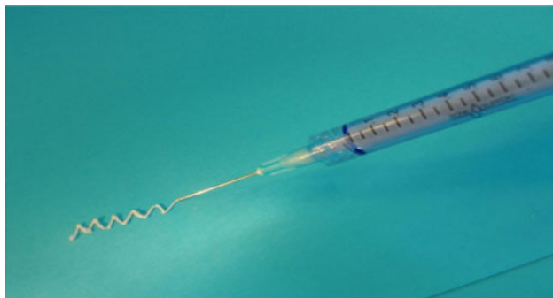
Fig. 1 Mixed paste of calcium sulphate/hydroxyapatite composite (Cerament™ SpineSupport) in a 1 mL syringe (23G needle)
