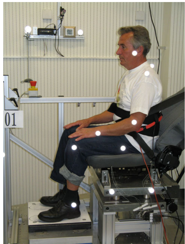
Fig. 2 Patient sitting on a driver seat fixed to a hexapod
