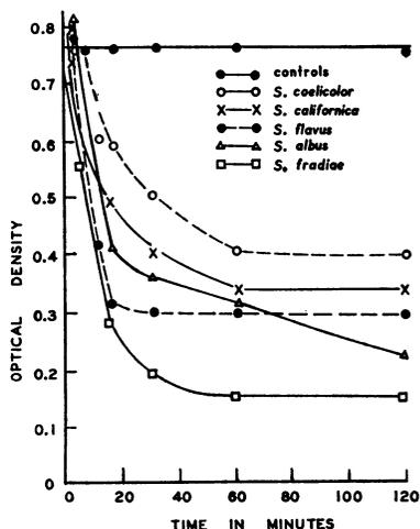
Figure 1. Lysis of Streptomyces cells by lysozyme, 100  $\mu$ g per ml in M/15 Sorensen's phosphate buffer, pH 6.6, containing 0.01 M sodium chloride; reaction carried out at 37 C.
