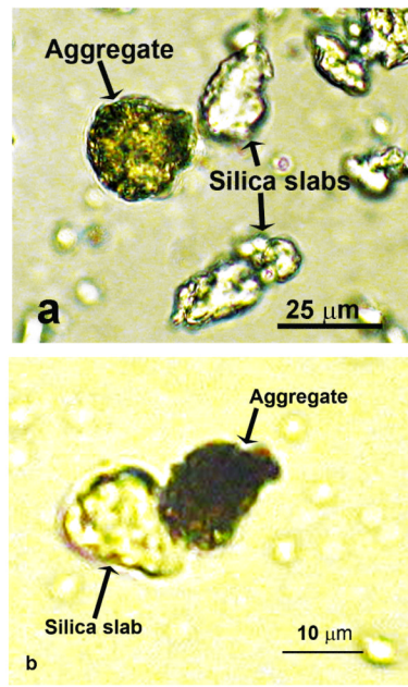
Figure 2. Spherical polybutadiene/silica aggregates (0.25:1) of size a: 25μm and b: 10μm and several irregular silica slabs, components of the complex filler used in this work.
