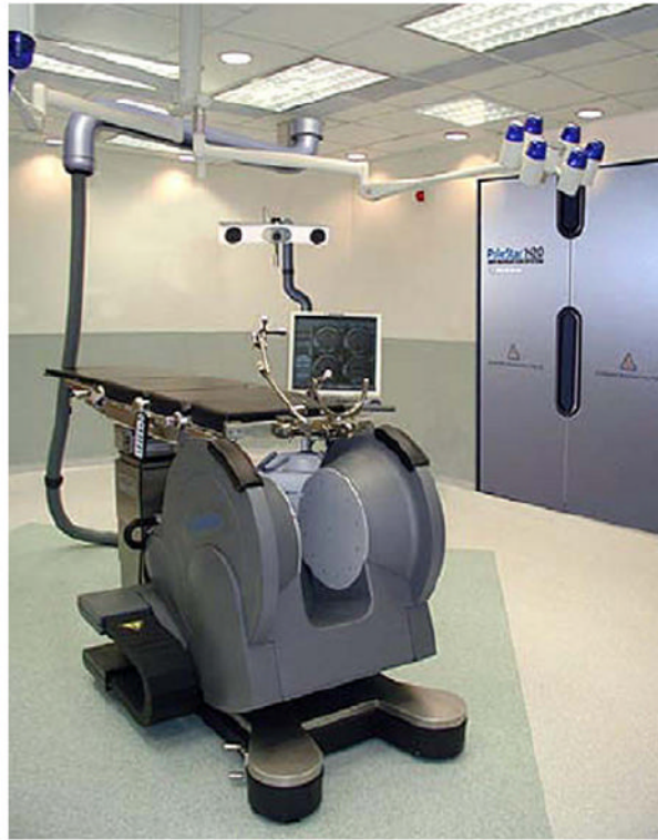
Fig. 4. The PoleStar iMRI. The open-bore configuration PoleStar N-20, despite its low-field 0.15T magnet, has allowed many institutions to take advantage of iMRI without completely remodeling their operative suite to accommodate a larger, high-field stationary iMRI. The Polestar is compact enough to be stored in a shielded room (pictured on the right side of the figure) when not in use. If a smaller room cannot be dedicated to storage, an in-suite “hangar” can be set up to shield the magnet when not in use. ( Courtesy of Medtronic Navigation, Louisville, CO; with permission. )
