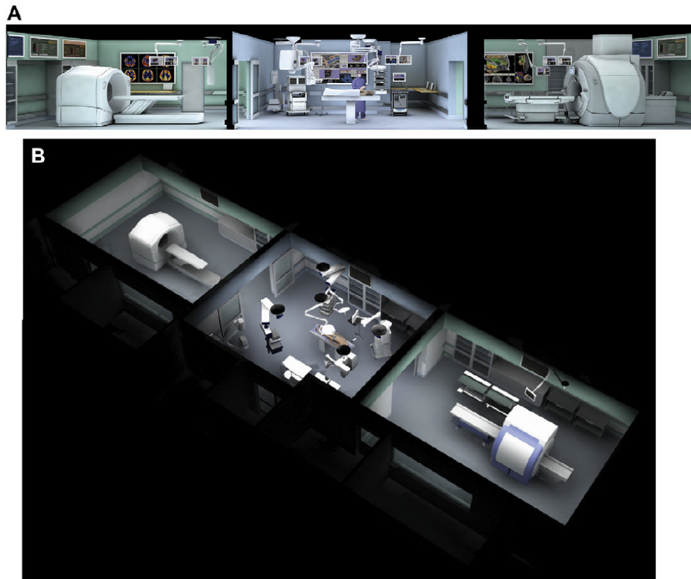
Fig. 7. The Advanced Multimodality Image Guided Operative (AMIGO) suite at the National Center for Image Guided Therapy, BWH and the Harvard Medical School. In AMIGO, real-time anatomic imaging modalities such as radiography and ultrasound are combined with the cross-sectional digital imaging systems of PET-CT and MRI. (A, B) Cross-sectional and oblique views of the three-room suite composed of a PET-CT (left room), state-of-the-art operating room, and 3.0T MRI (right room). (Courtesy of GE Healthcare, Wauwatosa, WI; with permission.)
