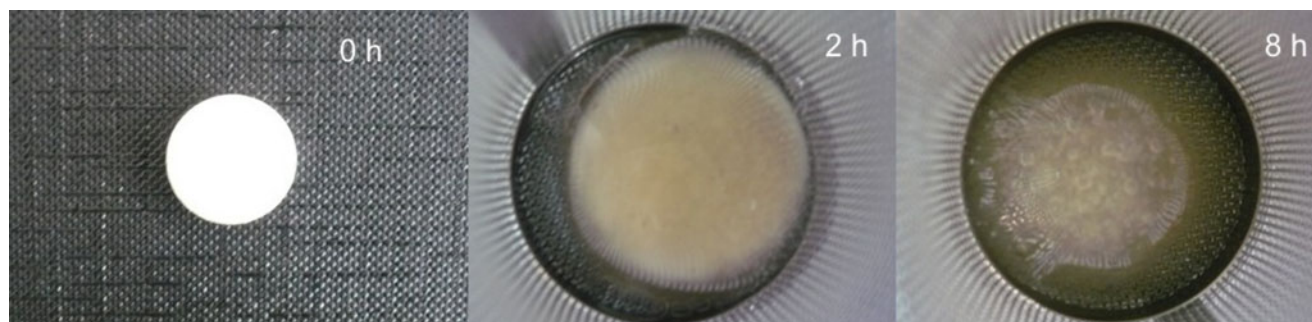
Fig. 9. The appearance of F2 formulation in dissolution media at time 0, 2, and 8 h
