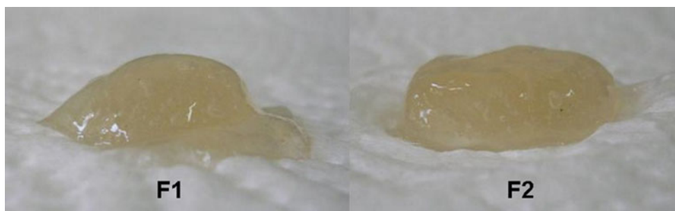
Fig. 10. Sideways cross-section of the swollen tablets of F1 and F2
