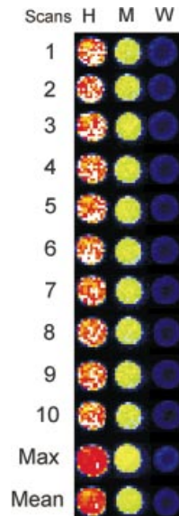
Figure 1. Variability of signal detection on microarray spots with multiple scans. A single microarray was subjected to 10 consecutive laser scans for Cy3 fluorescence. Three spots representing high (H), medium (M) and weakly expressed (W) transcripts were chosen, and the corresponding pixel regions obtained in the 10 images are shown in rows 1–10. Note that pixels with the same localisation within the spots often have different intensities. \Sigma POT software integrations of the 10 images are reported in rows 11 and 12. The image in 11 has been obtained using the highest intensity value of each pixel, while the image in 12 has been obtained by using the average intensities of each pixel among the 10 scans. The enhancement of spot intensity after both calculations is evident, especially for the low-intensity spot.
